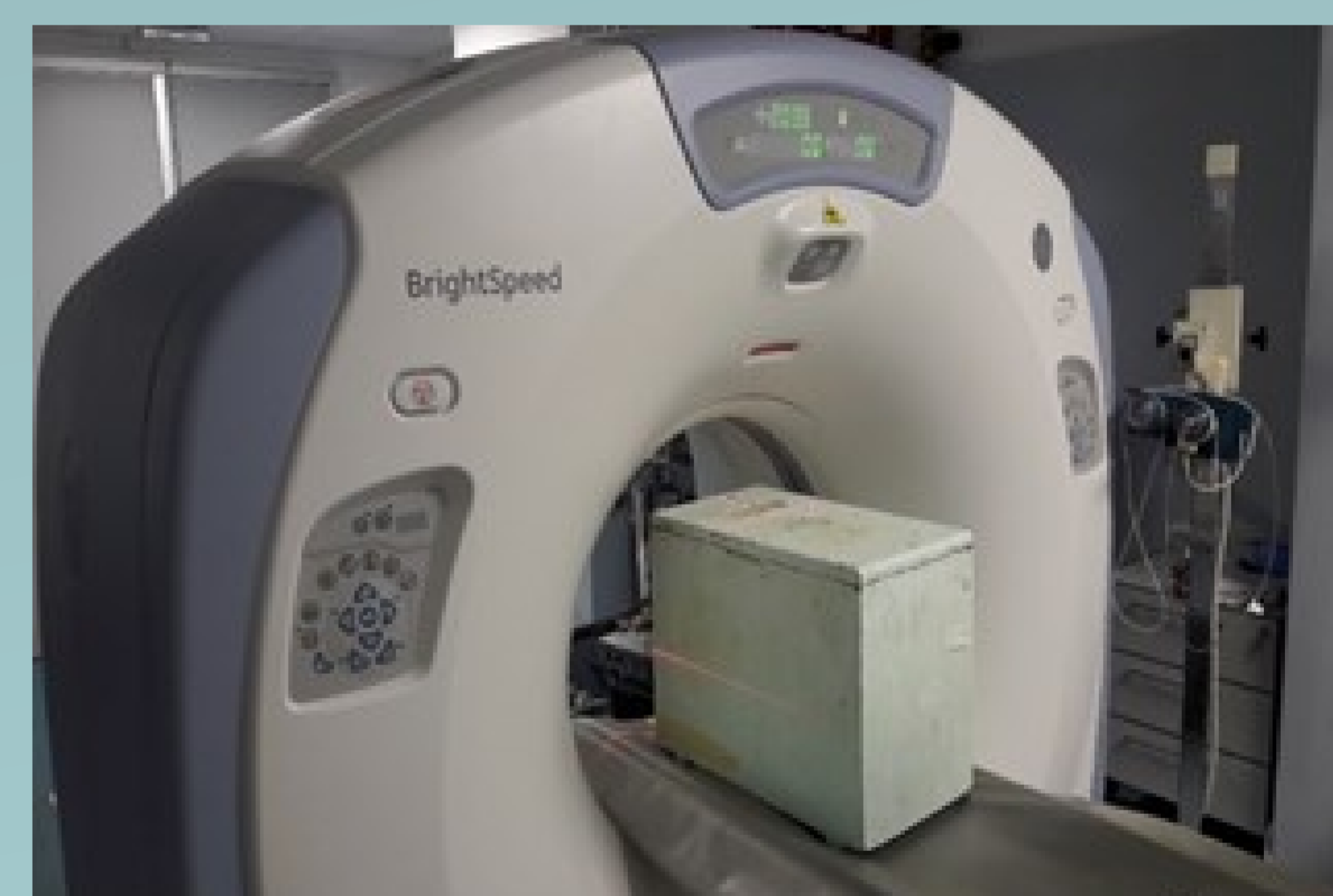
Figure 2. Computed Tomography examination of the brood combs temporarily inserted in a 6-frame polystyrene hive
